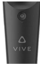
Figure 4.9: Turn on the controllers
