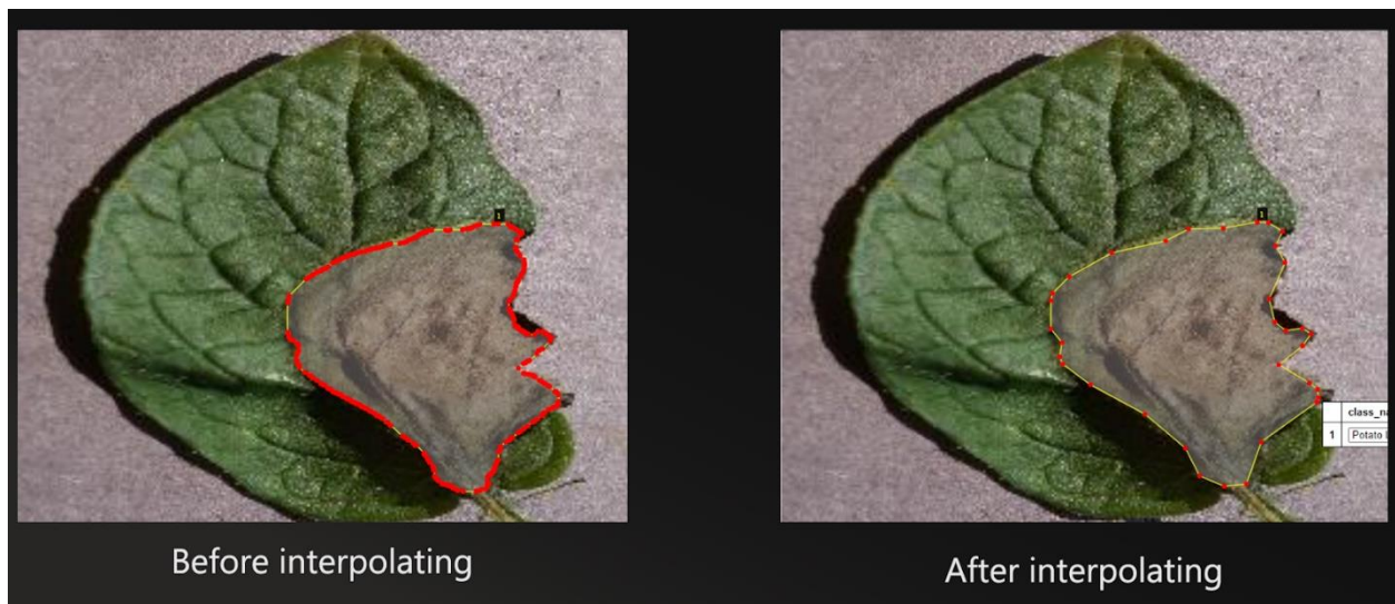
Figure 3.9: Reducing Polygon points using RDP
