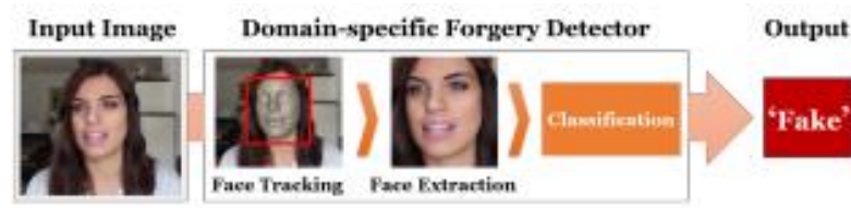
Figure-4: The capture picture is created using a trustworthy face-localization technique in which I utilized the fact that pick out the locale of a picture which is protected by confront. This area was then contribute to a trained categorization system to get the expected image. This is frequently the face modification domain-specific forgery detection process.
