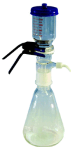
Figure 2: Filtration of extract Vacuum Filtration Apparatus
