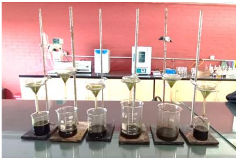
Figure 2: Filtration of extract via funnel with filter paper
