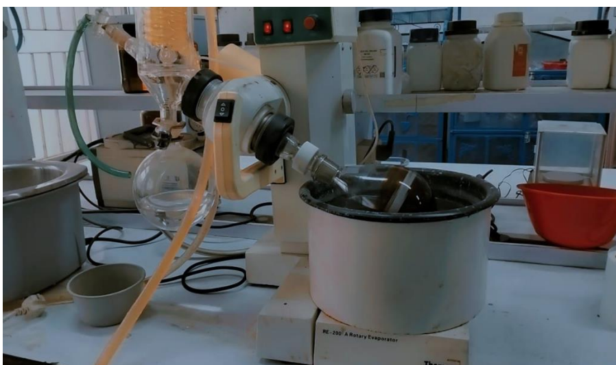
Figure 3: Evaporation of extract via Evaporator
