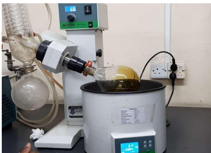
Figure-6: Evaporation of methanol from the liquid extract
