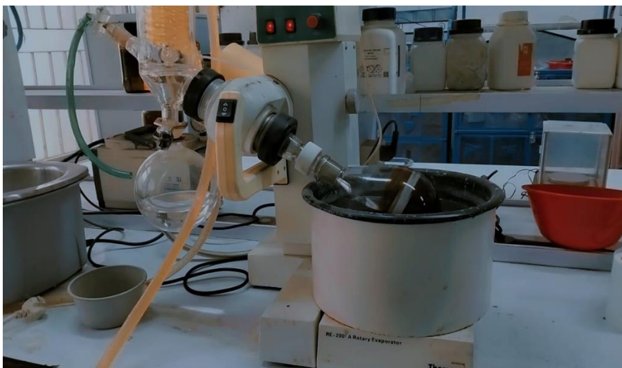
Figure 5: Evaporation of extract via Evaporator
