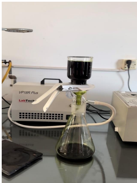
Figure 02: Vacuum filtration of Acmella Oleracea
