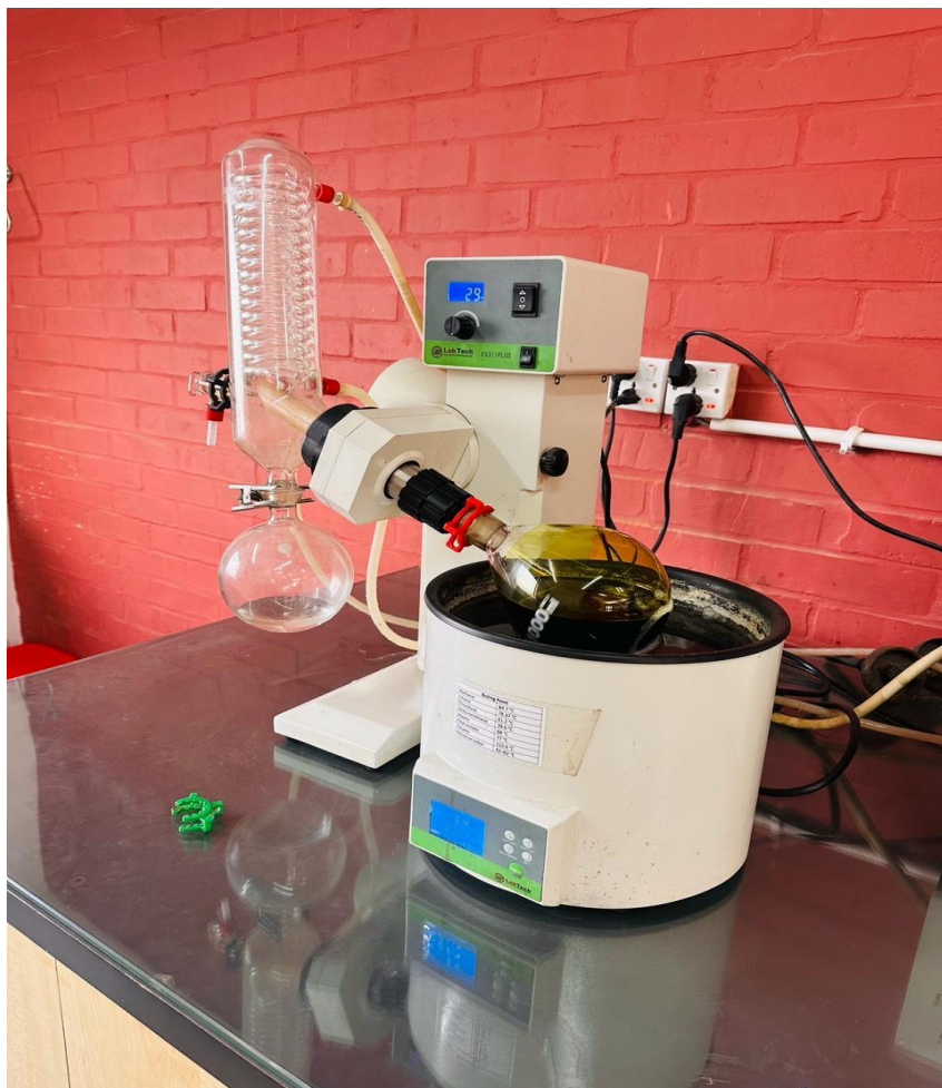
Figure 04: Rotary Evaporation of Acmella Oleracea
