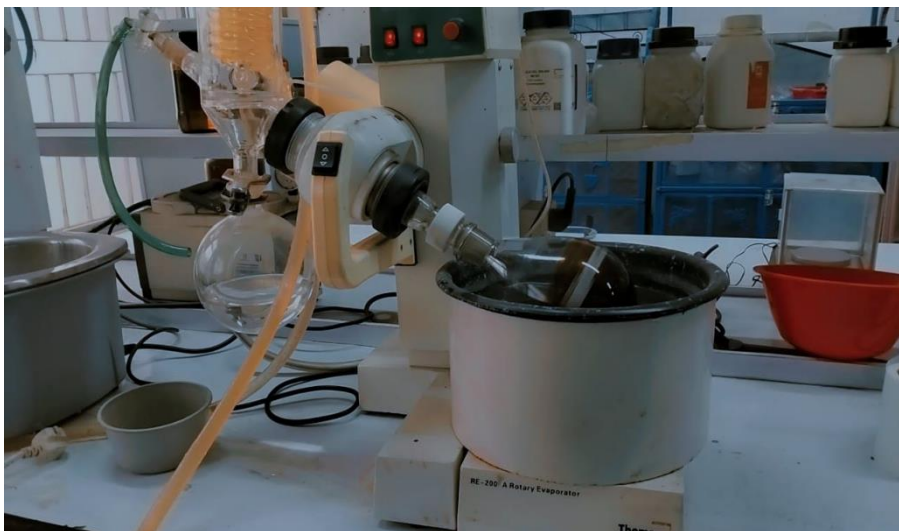
Figure 3: Evaporation of extract via Evaporator
