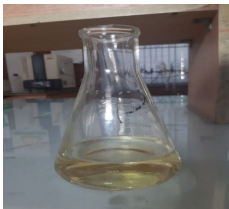
Figure 10: Titration endpoint in light yellow
