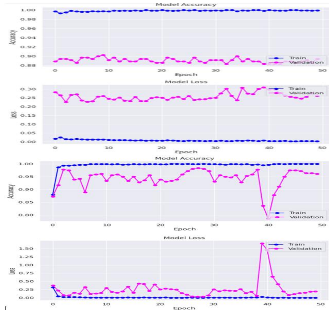
Figure 5.3.1: Training and validation accuracy and loss over the epochs VGG16 & EfficientNet Transfer Learning
