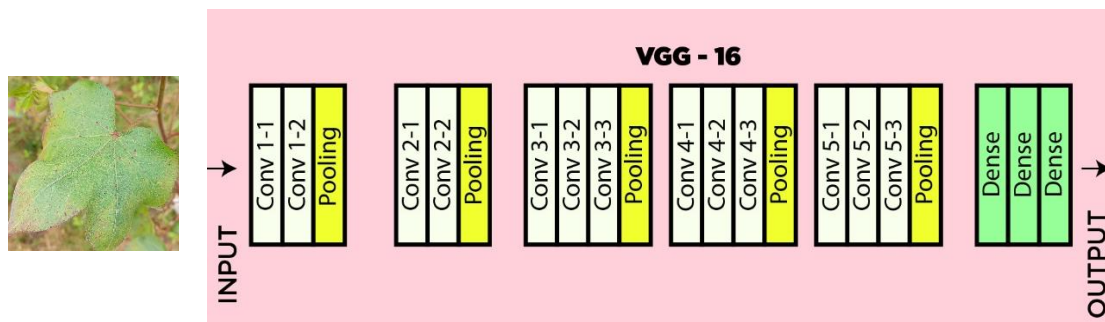
Figure 3.2.3: The proposed Model Architecture (VGG16, Source: google modified)
