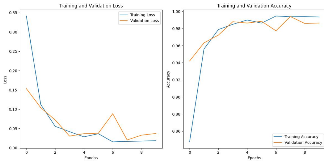
Figure 5.3: Training and validation accuracy and loss over the epochs (Xception)
