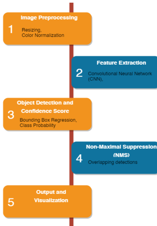
Fig 3.1 Proposed Methodology Diagram
