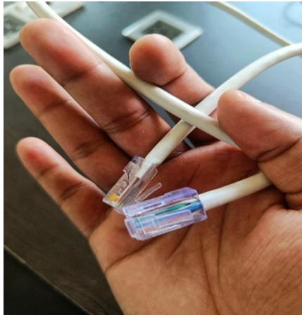
Figure 3.4: Put CAT 6 cable into RJ45 connector
