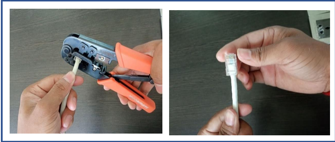
Figure 3.3.2 Insert RJ-45 Connector twisted pair cable
