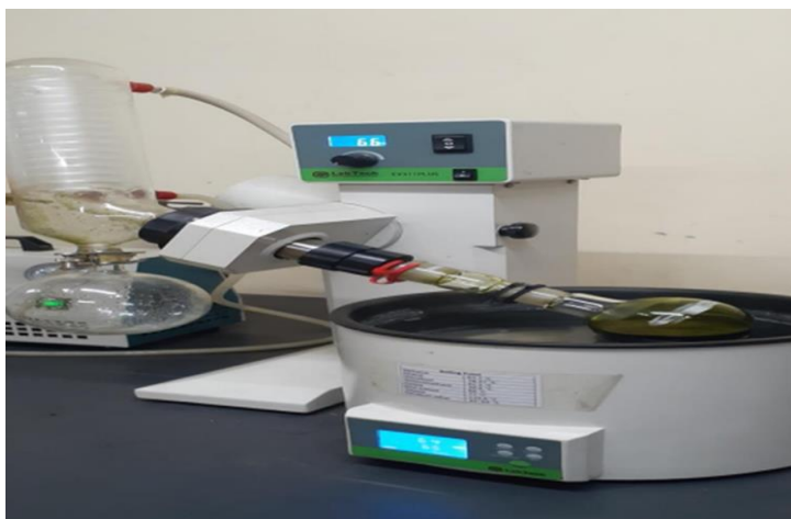
Figure 5: Evaporation of extract via Evaporator
