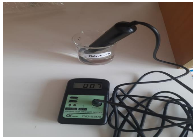
Fig 3.12: Testing DO in the lab
