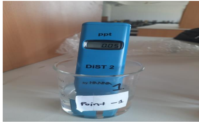
Fig 3.8: Testing Electrical Conductivity in the lab
