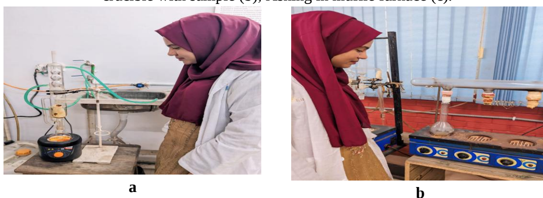
Figure 6: Extracting fat using Soxhlet apparatus (a), Sample digestion in kjeldahl apparatus (b).
