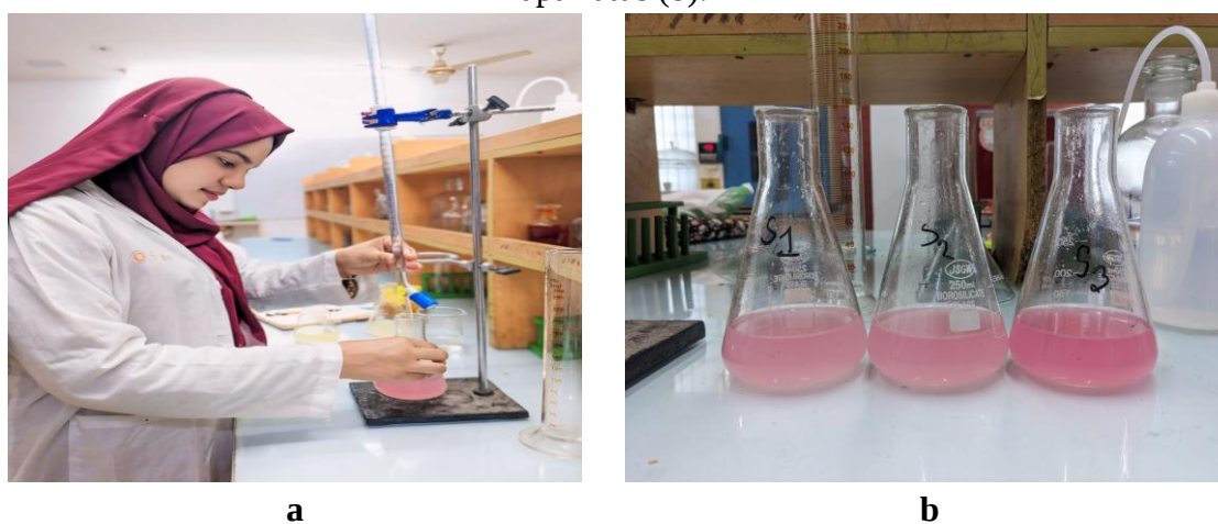
Figure 7: Titration with NaOH (a), Titration endpoint color changed (b).
