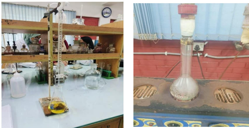
Figure 5: Kjeldahl method for protein analysis
