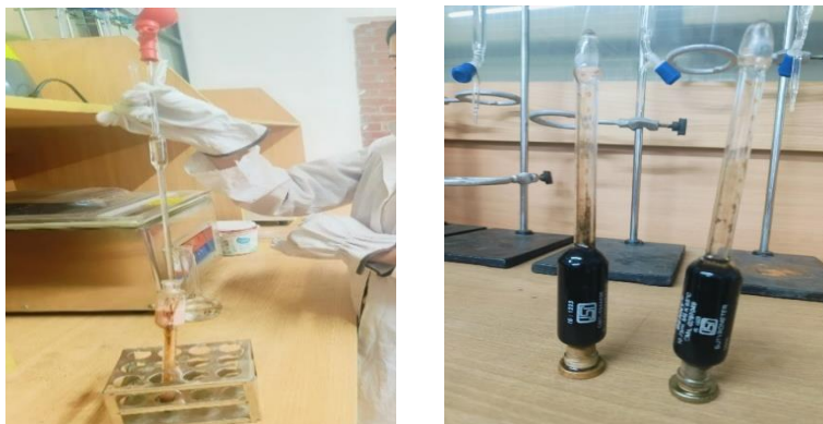
Figure 4: Garber test procedure for fat analysis
