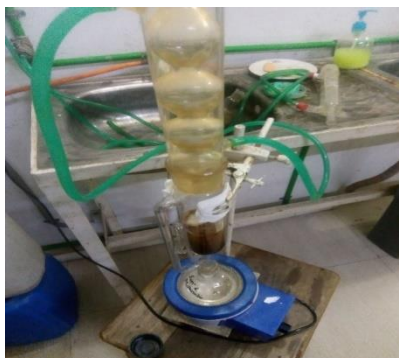
Figure No:6 Extraction of fat by Soxhlet apparatus
