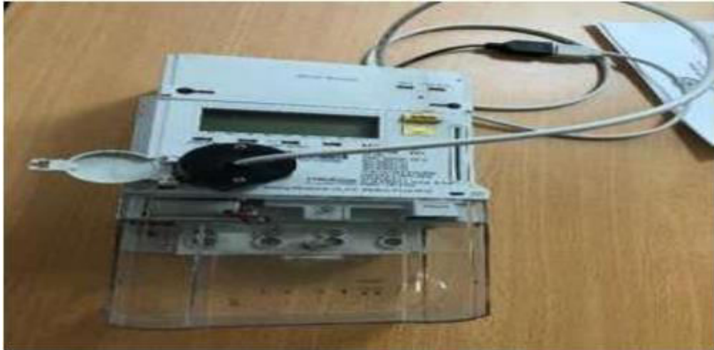
Figure6.6: Smart Card System Prepaid Meter
