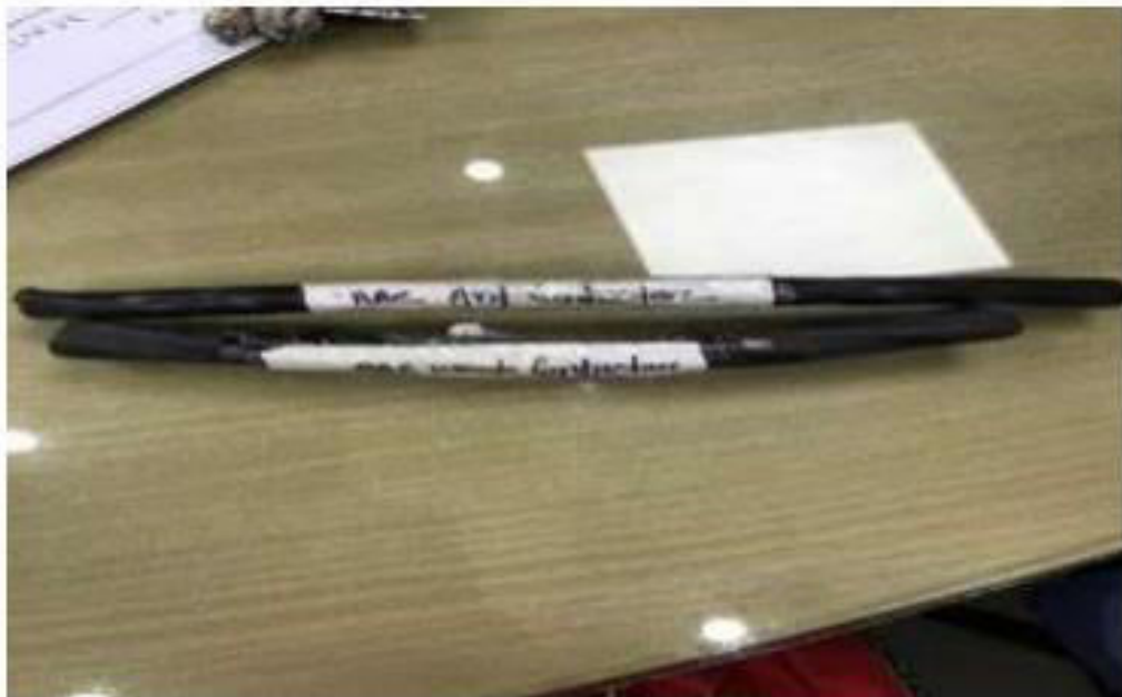
Figure 6.1: 0.415 KV line over heads wires
