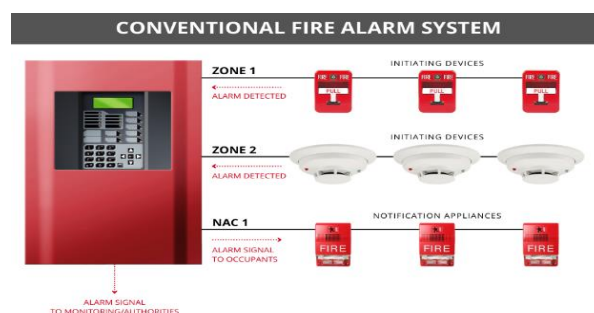
Figure 3.1: Conventional Fire Alarm System.
