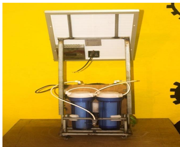
Fig 3.3.1: Water Purification Unit
