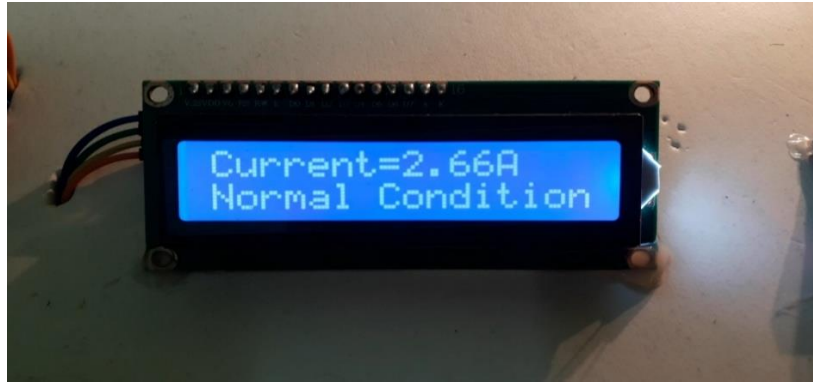
Fig. 4.4: Normal Condition with Two Load On
