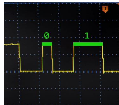
Figure-6: DHT22 Voltage magnitude count as Binary 0 or 1.
