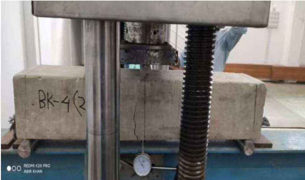
Figure 4.8.9: Failure Pattern (for Type 4-2 Beam)
