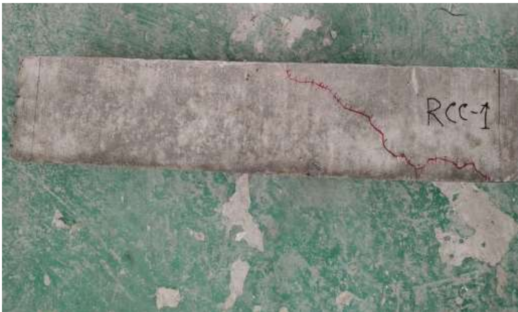
Figure 4.8.4: Failure Pattern (for Type 2-1 Beam)
