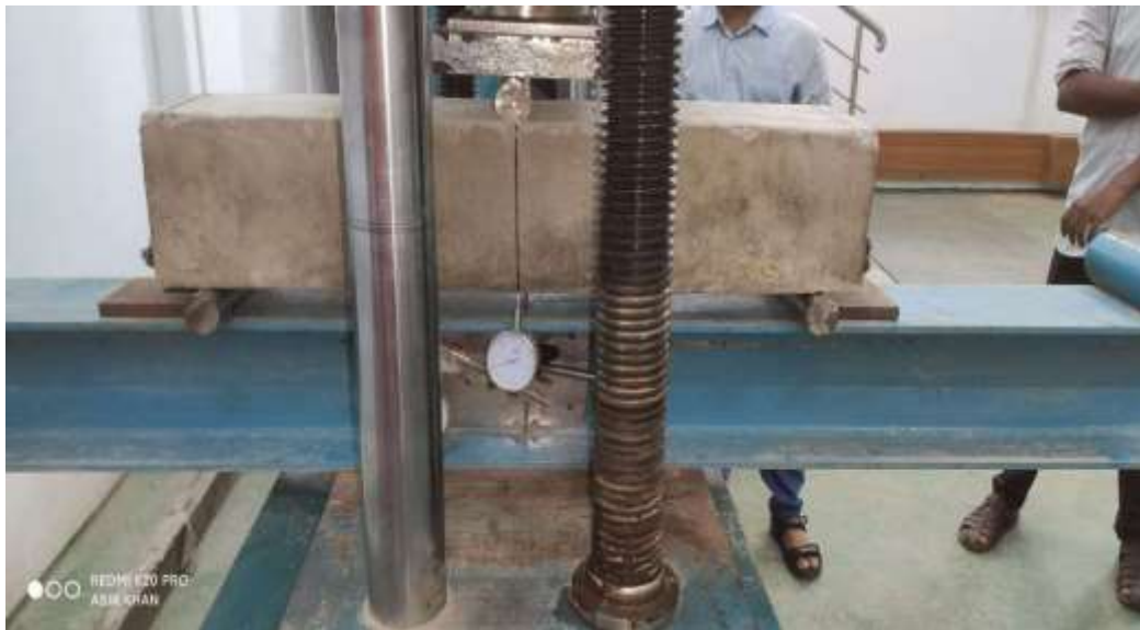
Figure 4.8.2: Failure Pattern (for Type 1-1 Beam)
