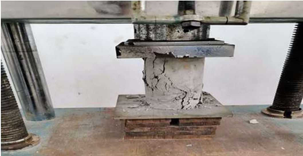
Figure: 3.6.1: Compressive Strength Test for Slender
