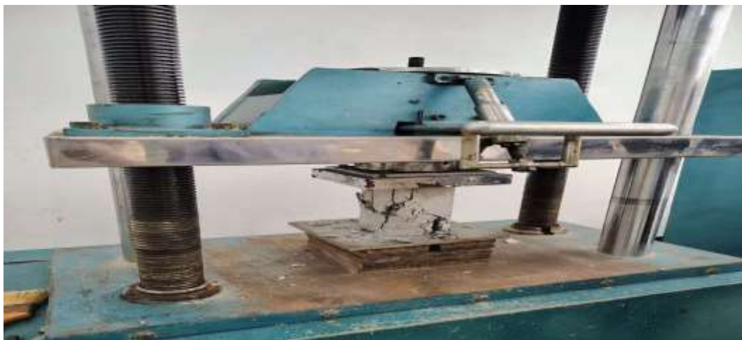
Figure: 3.6.2: Compressive Strength Test for Slender
