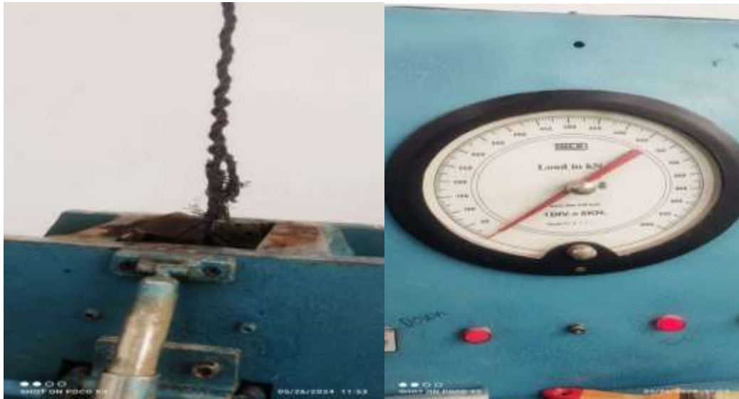
Figure 3.7.2: Textile Fabric Reinforcement Tensile Strength Test
