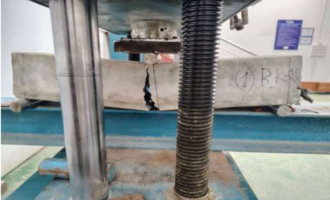
Figure 3.9.6: Beam Setup for Test
