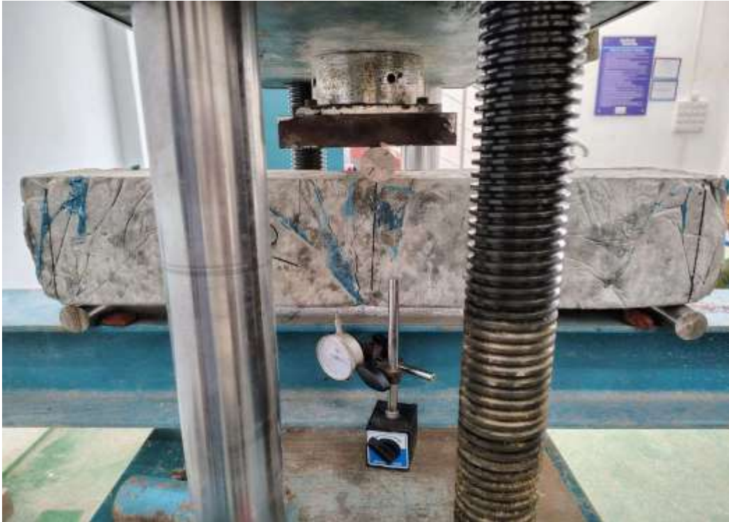
Figure 4.8.3: Failure Pattern (for Type 1-2 Beam)
