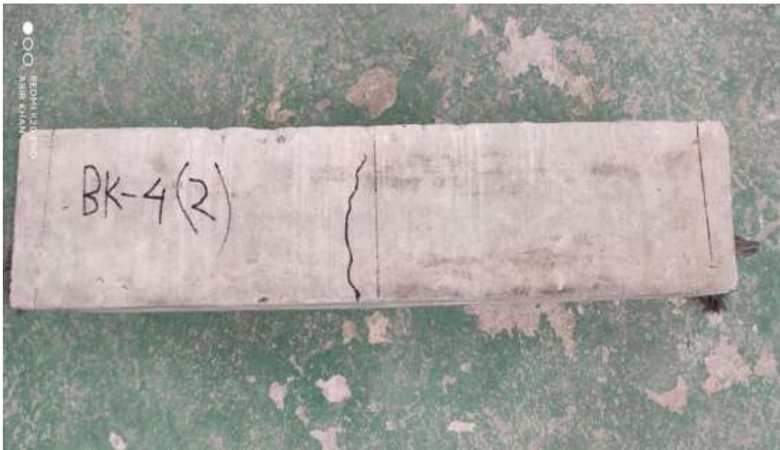
Figure 4.8.8: Failure Pattern (for Type 4-1 Beam)
