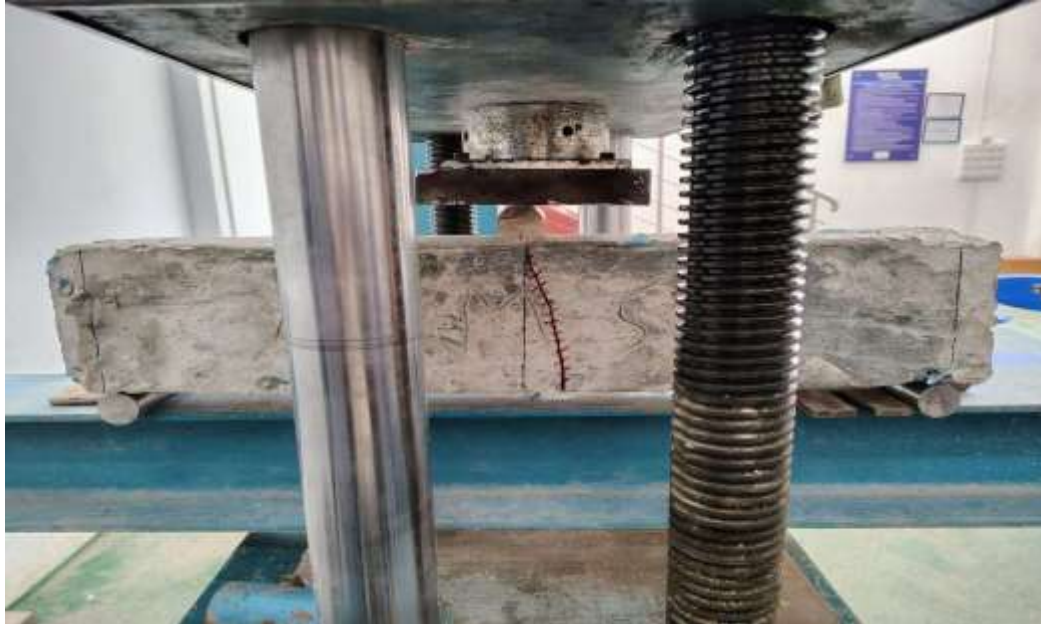
Figure 4.8.1: Failure Pattern (for Type 1-1 Beam)
