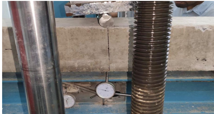
Figure 3-17: Reinforcement beam setup for test
