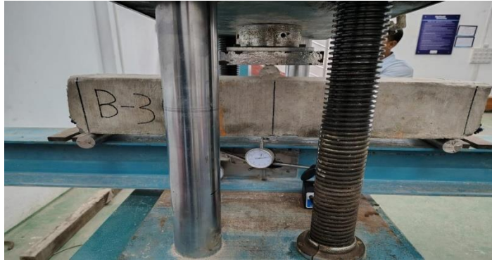
Figure 4-18: Cotton fiber beam setup for test
