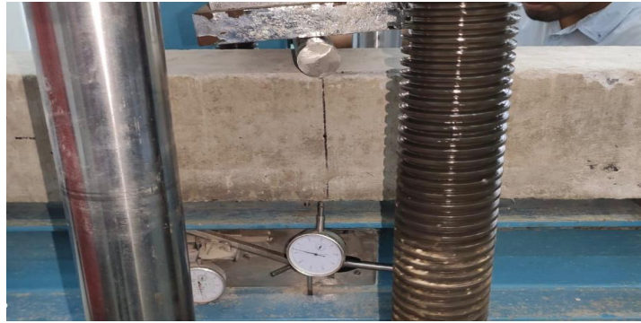
Figure 3-16: Pure concrete beam setup for test
