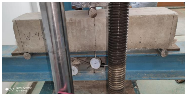
Figure 3-18: Nylon fiber beam setup for test
