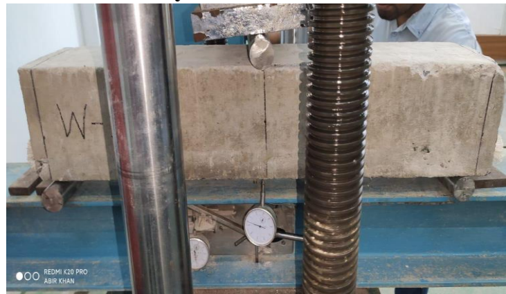
Figure 4-30: Nylon fiber beam setup for test
