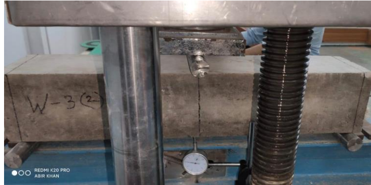
Figure 4-24: Nylon fiber beam setup for test
