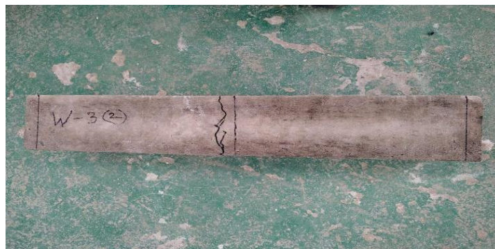
Figure 4-25: Failure pattern (Nylon fiber beam)
