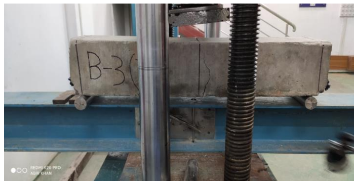
Figure 4-19: Failure pattern (cotton fiber beam)
