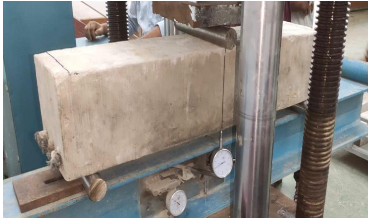
Figure 4-42: Polyester fiber beam setup for test
