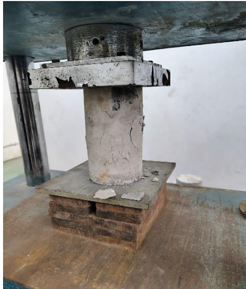
Figure 3-14: Concrete under compressive load
