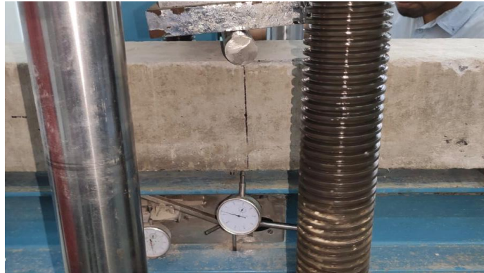
Figure 4-1: Pure concrete beam setup for test
