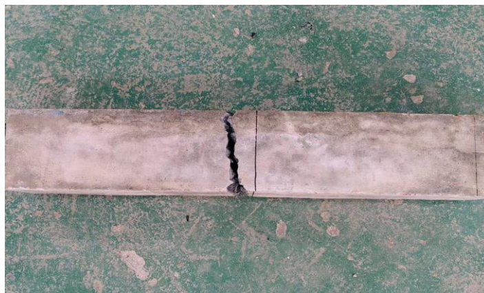
Figure 4-2: Failure pattern (Pure concrete beam)
