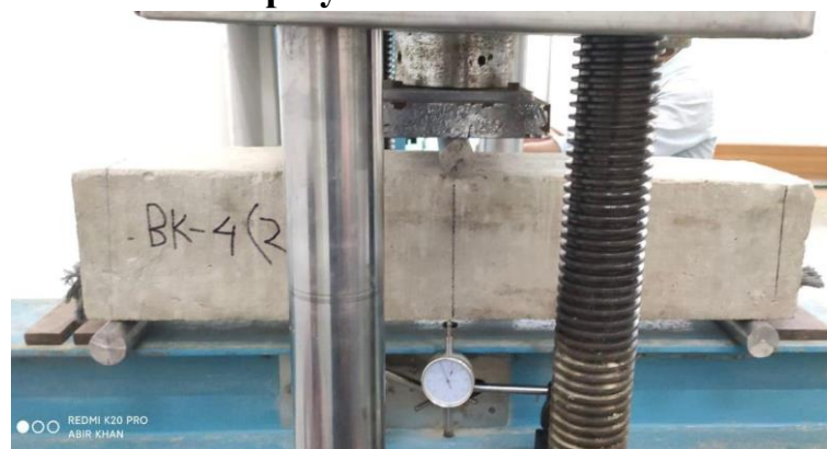
Figure 4-36: polyester fiber beam setup for test
