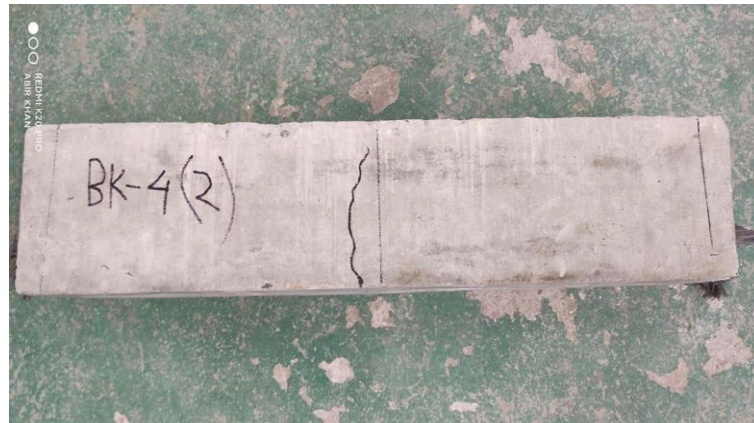
Figure 4-37: Failure pattern (Polyester fiber beam)
