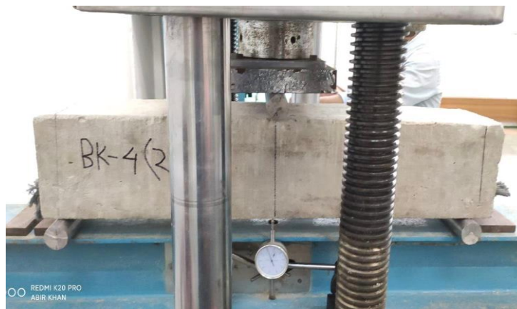
Figure 3-19: Polyester fiber beam setup for test
