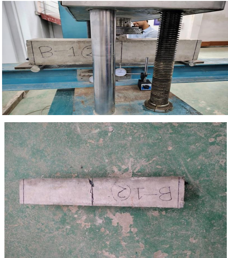
Figure 4-13: Cotton fiber beam setup for test
