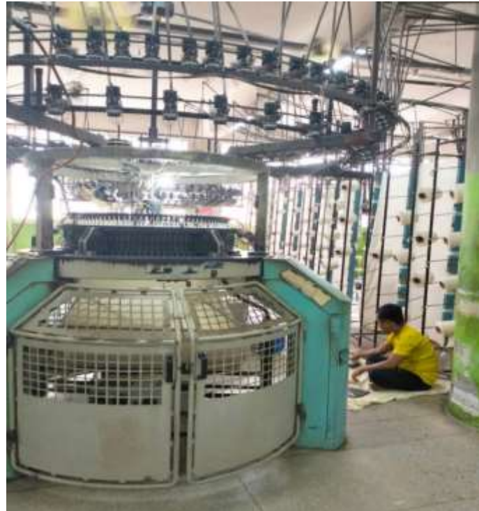
Figure 8: S/Jersey Circular Knitting Machine
