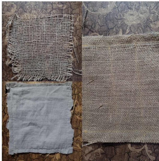
Figure-06: Single Layer Jute (Before & After Wash)
