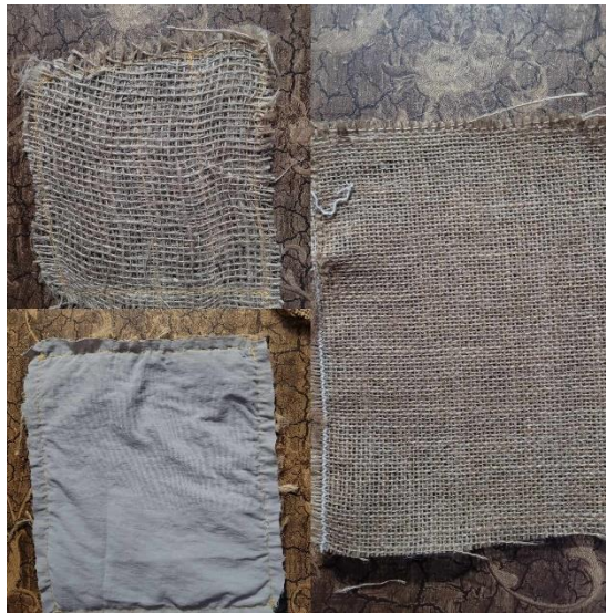
Figure-07: Double Layer Jute (Before & After Wash)
