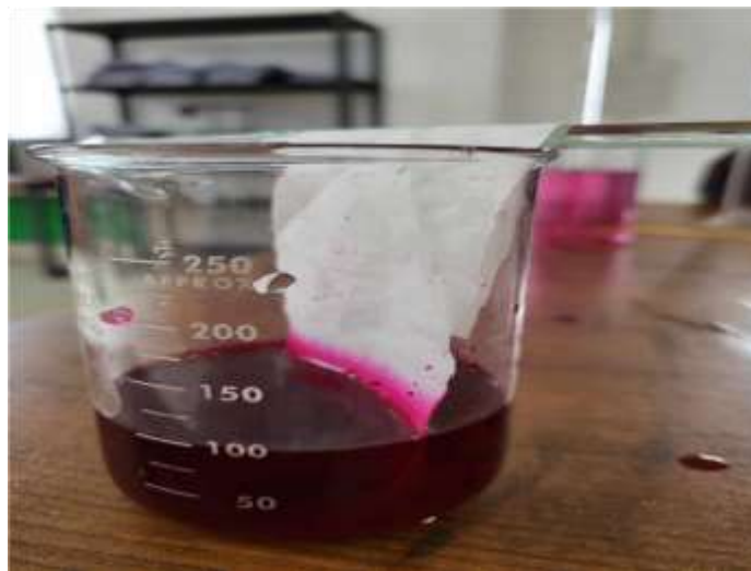
Figure:4.2:Wicking test report(After Using re-use bath)
