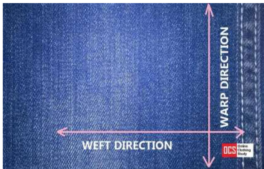
Figure 3: Warp and weft yarn in fabric
