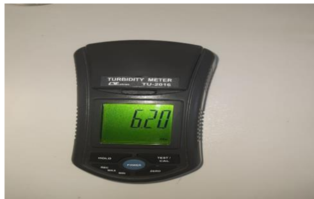
Fig 3.8: Testing Turbidity in the lab
