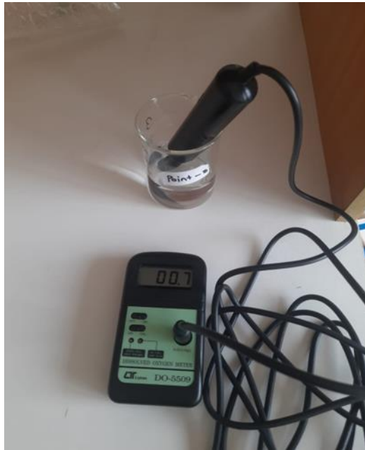
Fig 3.11: Testing DO in the lab
