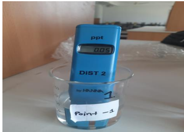
Fig 3.7: Testing Electrical Conductivity in the lab
