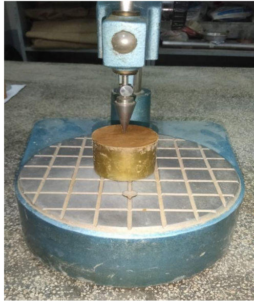
Figure 3-11: Testing with cone penetrometer
