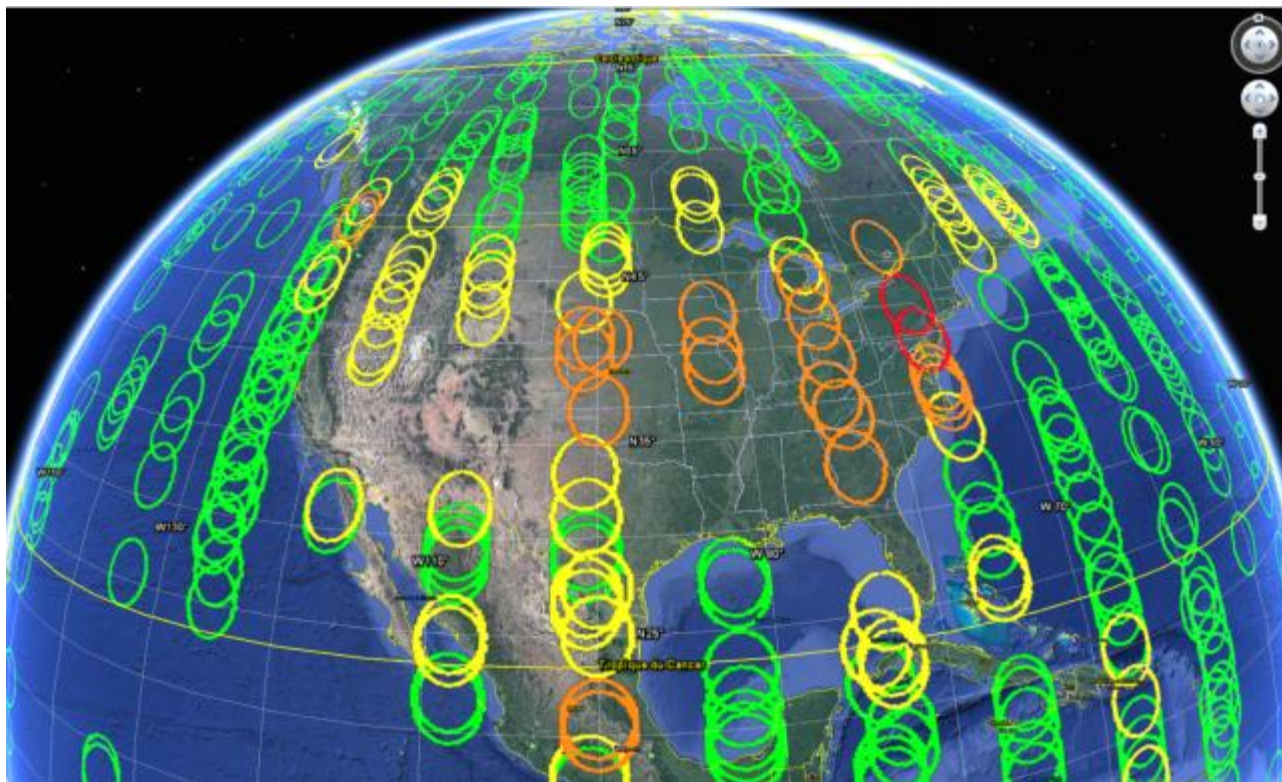
Locations of spot beams simulated over the northern part of Region 2. Green beam: fewer than 50 aircraft in the area. Yellow beam: between 50 and 100 aircraft. Orange beam: between 100 and 400 aircraft. Red beam: more than 400 aircraft
