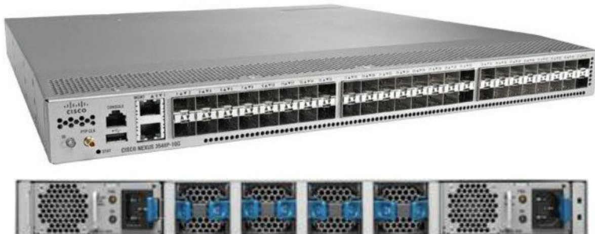
Figure 5, Cisco Nexus 3548-X Switch
