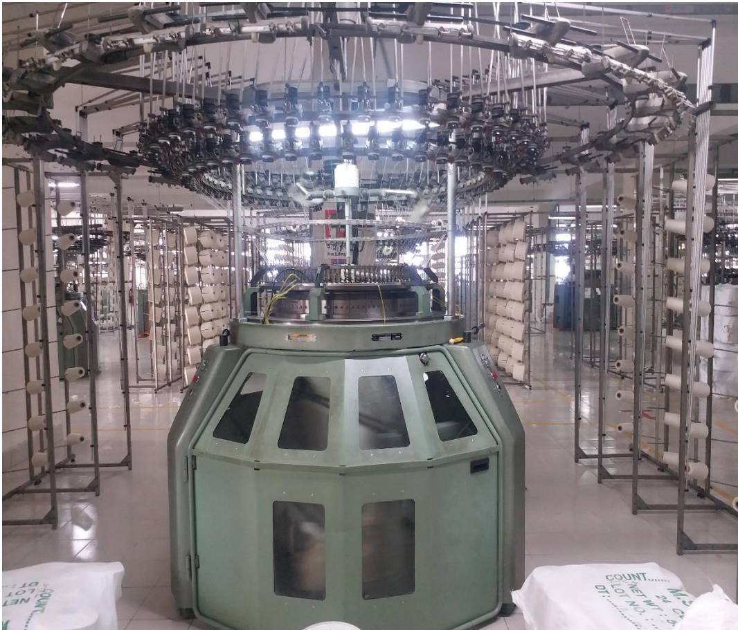
Fig 3.1.1: Single jersey circular Knitting M/C in knitting section.
