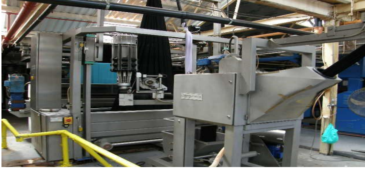
Figure 3.5.6 Corino Slitting & Dewatering Machine (For Open Width Fabric)
