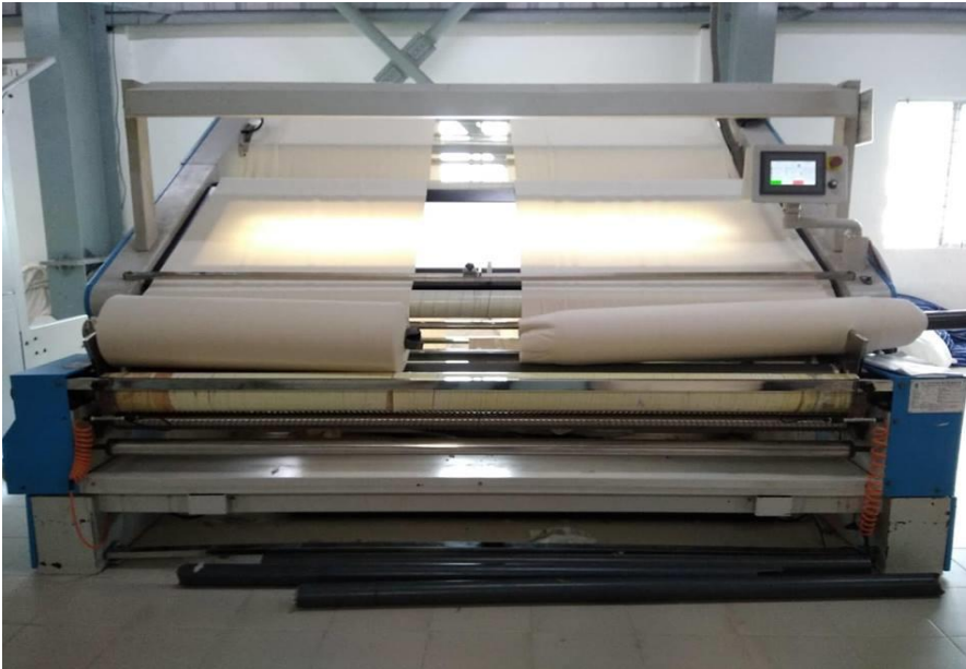
Picture: 3.2.19.1 fabric inspection
