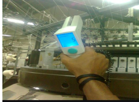
Figure 3.2.14.1: Measurement with stitch length meter
