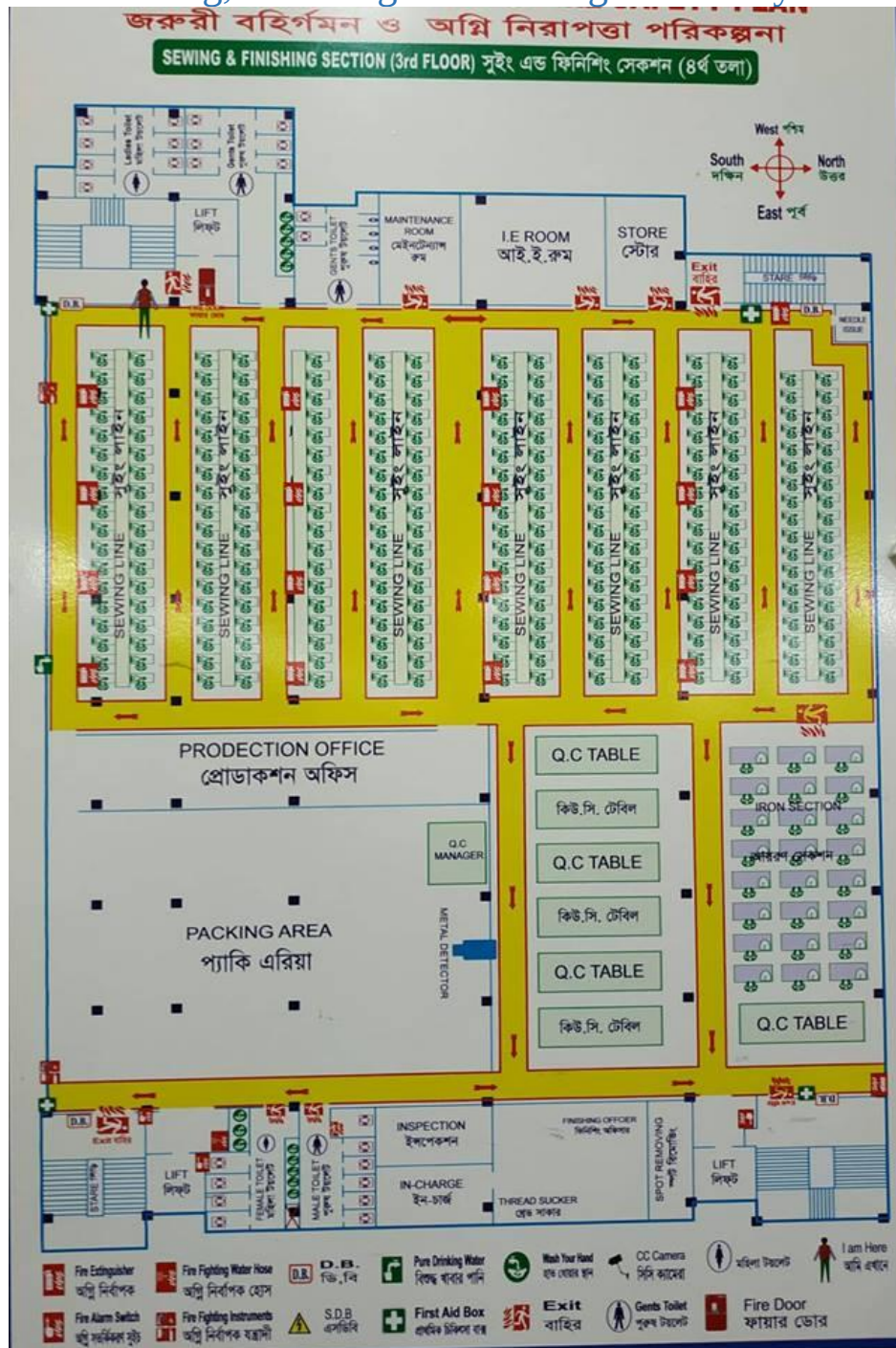
FIGURE3. 5 SEWING, FINISHING AND PACKING SECTION LAYOUT
