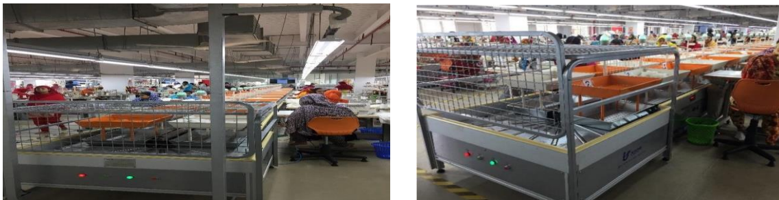
Figure 3. 7. 3 Conveyor sewing line
