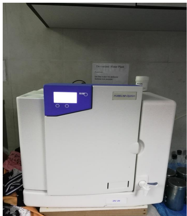
Figure: De-ionized Water Plant
