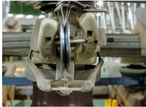
5.KNOT CATCHER: It detects the knot in the yarn and cut.
