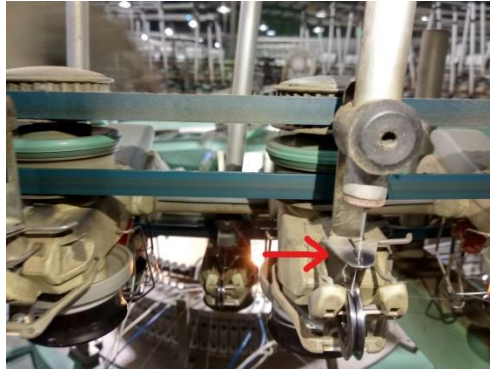
6.VDQ PULLEY: It control the stitch length & GSM of fabric
