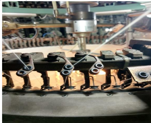
7.FEEDER: it helps the yarn to feed into the machine.
