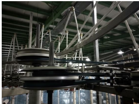
7.FEEDER: it helps the yarn to feed into the machine.
