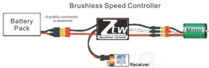
Fig 2.3.3 : ESC Connection Diagram
