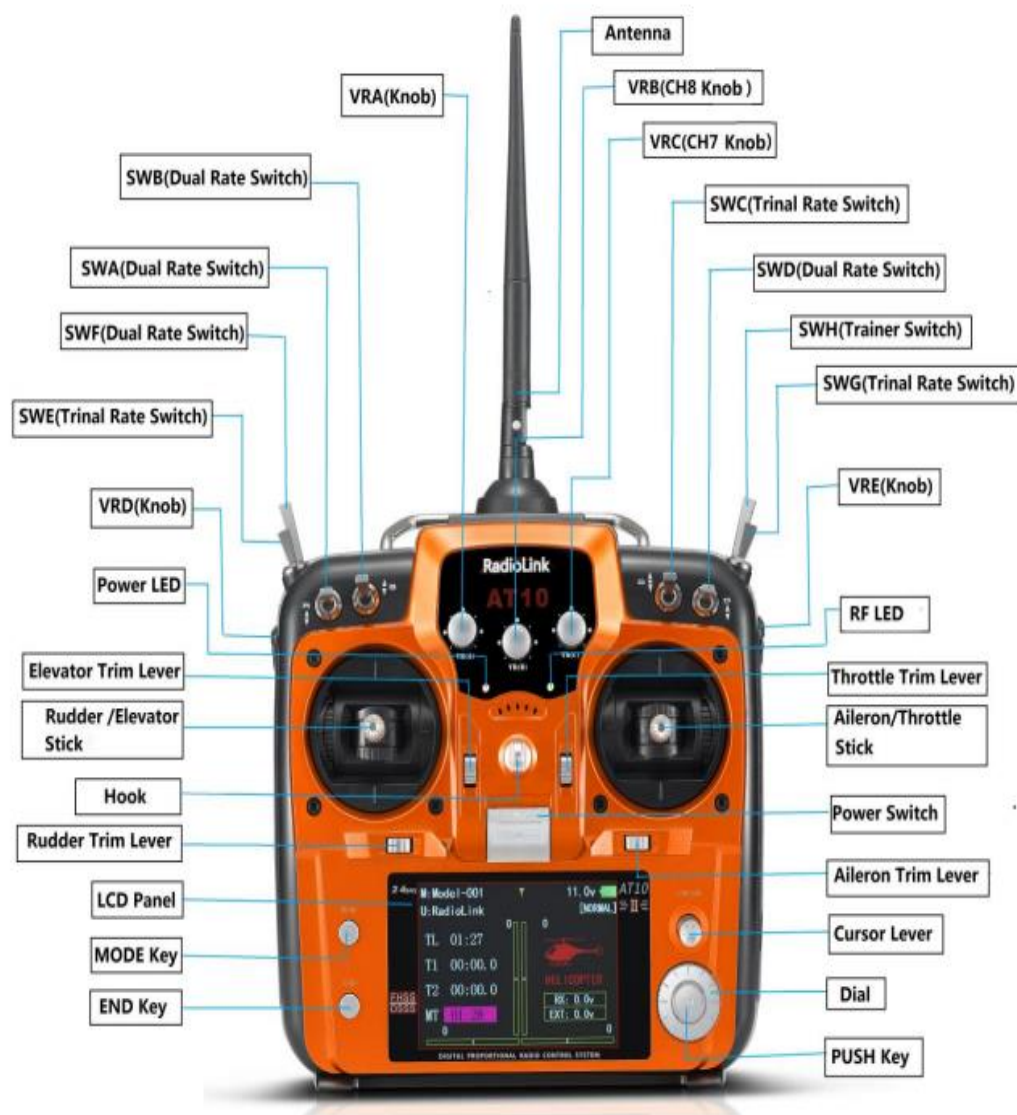
Fig 2.6.2 : Identify Font Part,Stick and Switch name of Transmitter
