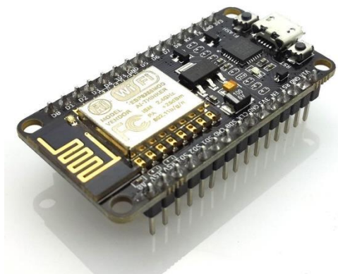
Figure 4.1: ESP8266 Node MCU Wi-Fi Module
