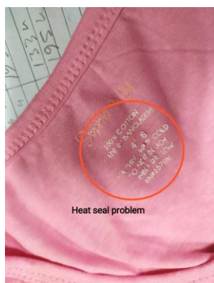
Fig: 2.10 Heat seal fault
