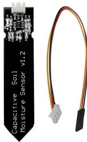
Figure 4.12: Capacitive Soil Moisture Sensor as a replacement
