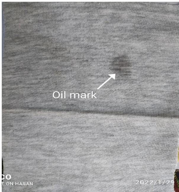
Fig. 13 Fault- Oil Mark.
