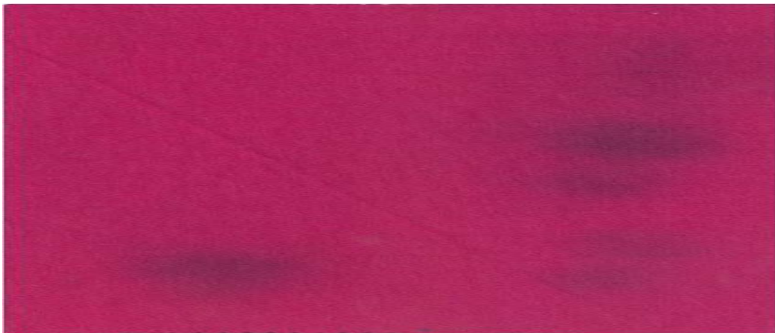
Fig. 3. Faults Name: Dye Spots.
