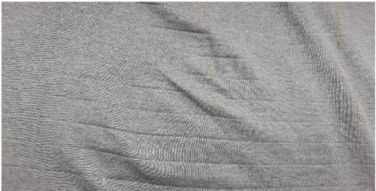
Fig. 17. Lycra Out Fabric construction: - 97/3 1×1 Rib Fault: - Lycra out
