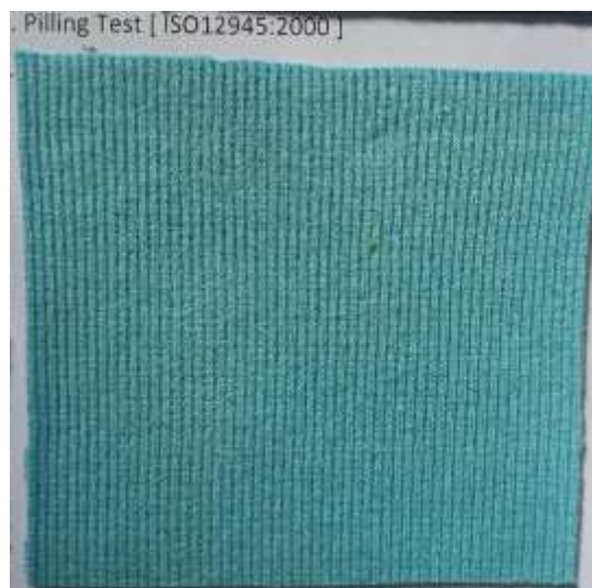
Figure 4.20: Result of turquoise pilling test
