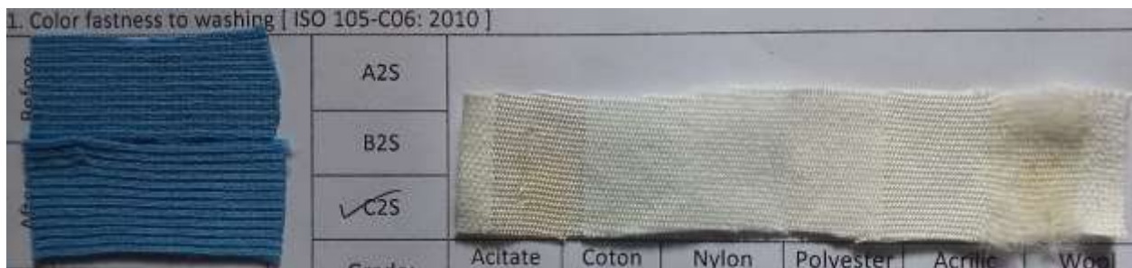
Figure 4.22: Result of Normal multi-fiber color fastness to Wash
