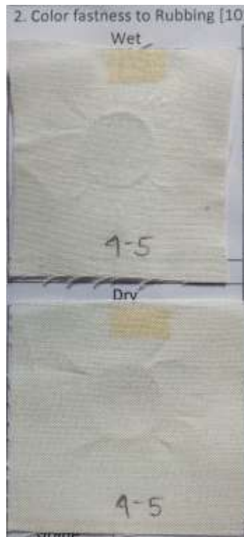
Figure 4.23: Result of Normal multi-fiber color fastness to Rubbing
