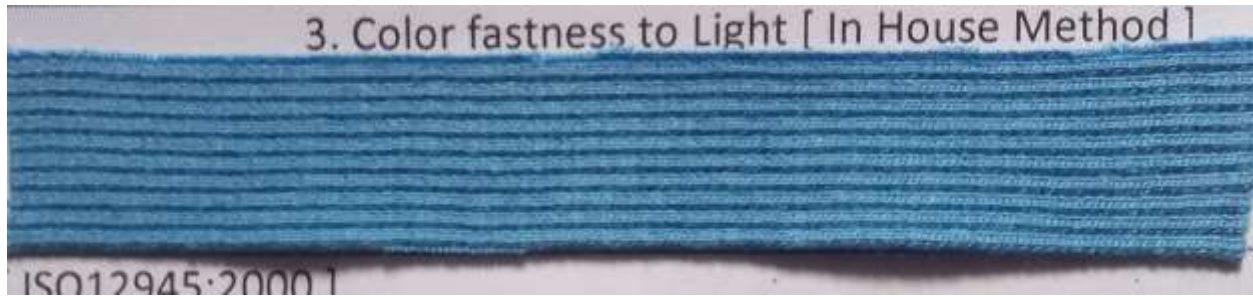
Figure 4.24: Result of Normal color fastness to Light
