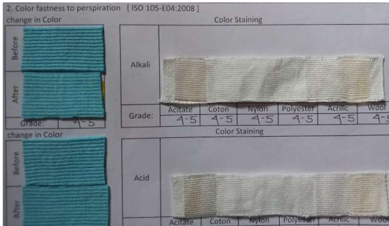
Figure 4.21: Result of Turquoise multi-fiber color fastness to perspiration
