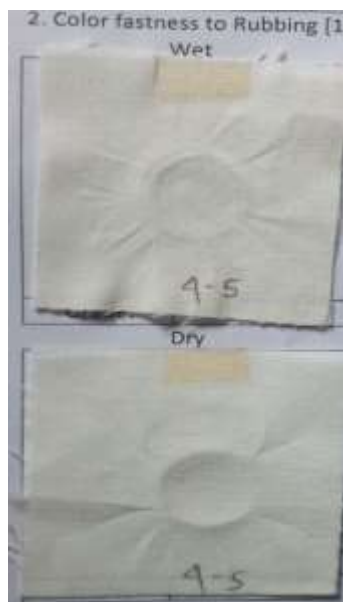
Figure 4.18: Result of turquoise color fastness to Rubbing
