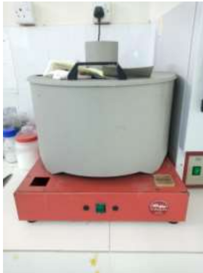
Figure 3.15: Color fastness to light (in house Method)
