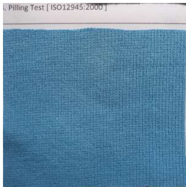
Figure 4.25: Result of Normal color Pilling test
