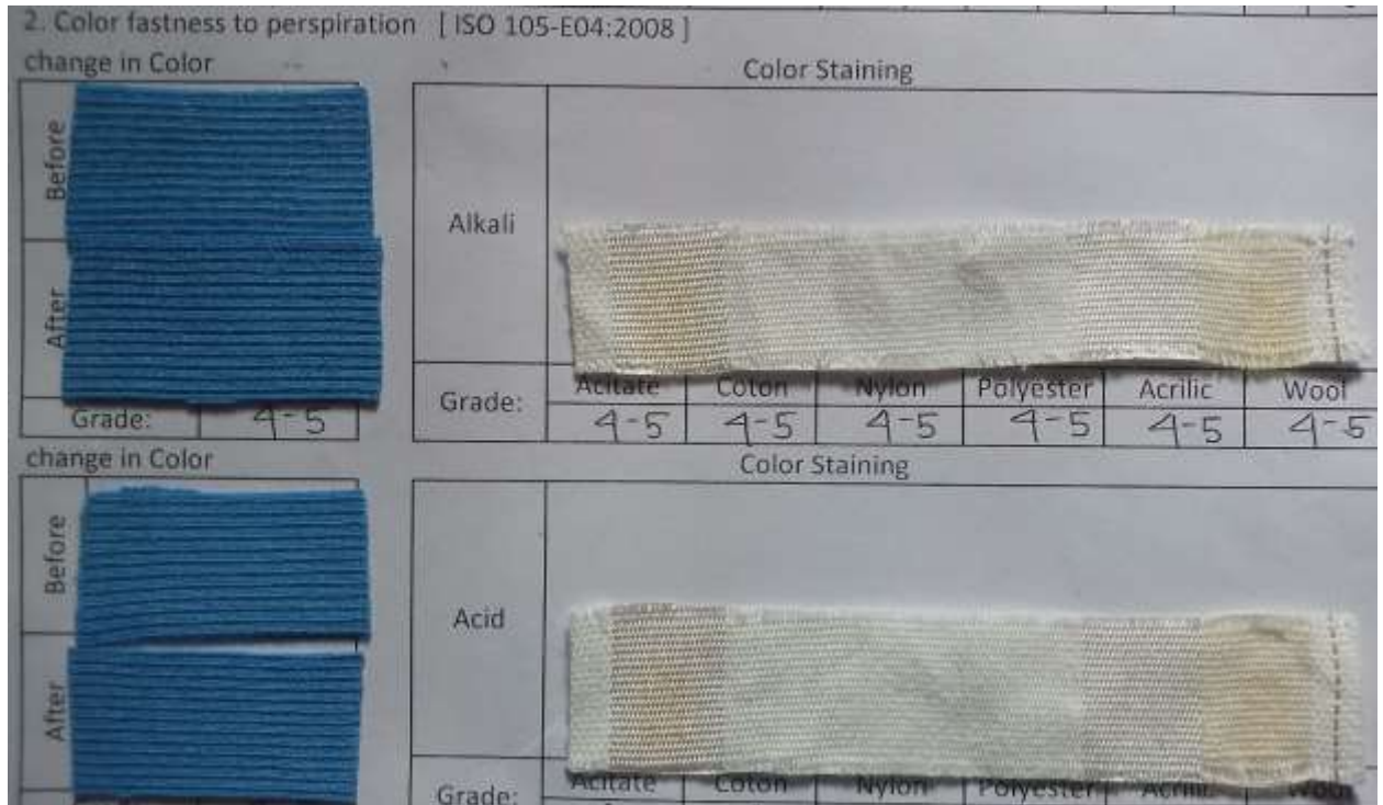
Figure 4.26: Result of Normal multi-fiber color fastness to Perspiration
