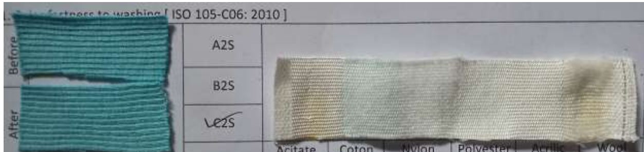
Figure 4.17: Result of turquoise multi-fiber color fastness to wash
