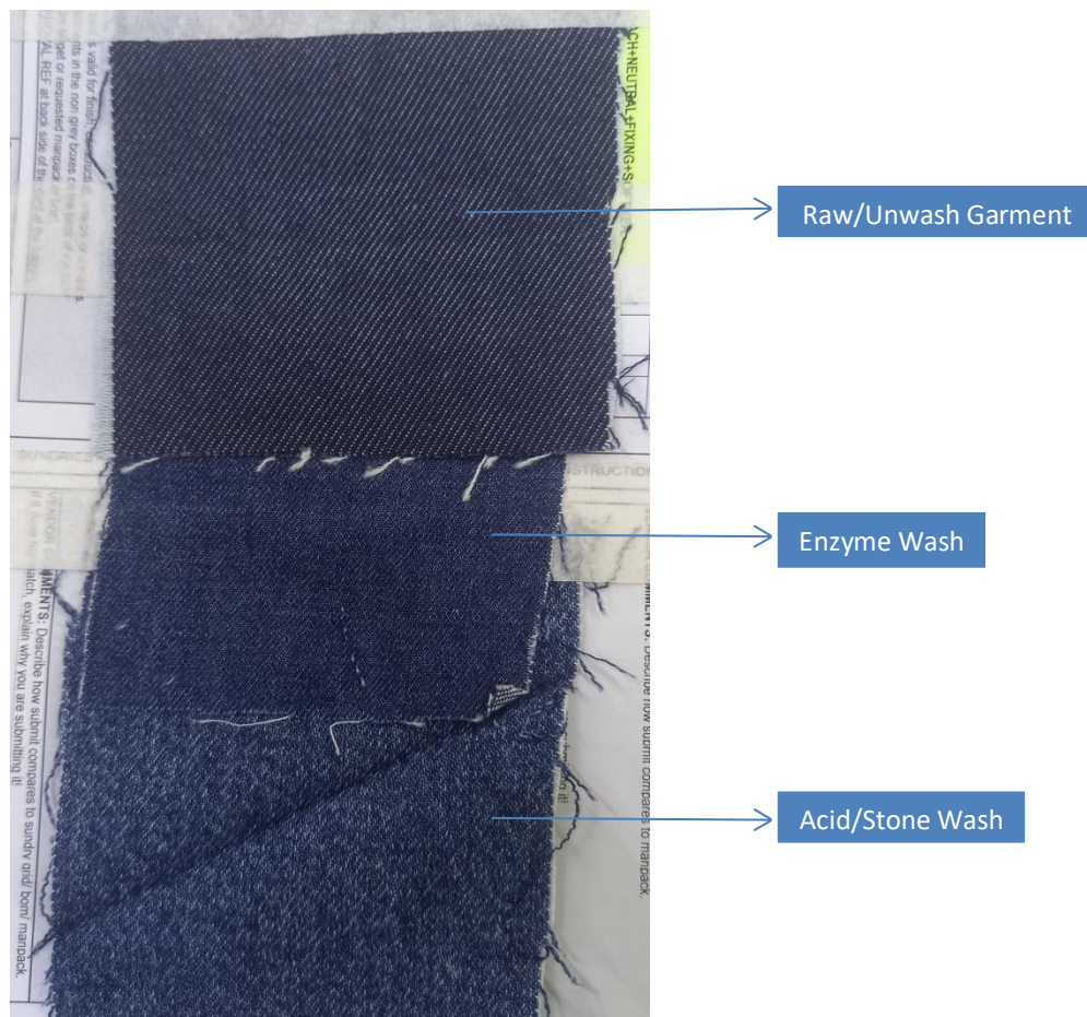
Figure: 3.6 Raw/Unwash & Acid Wash
