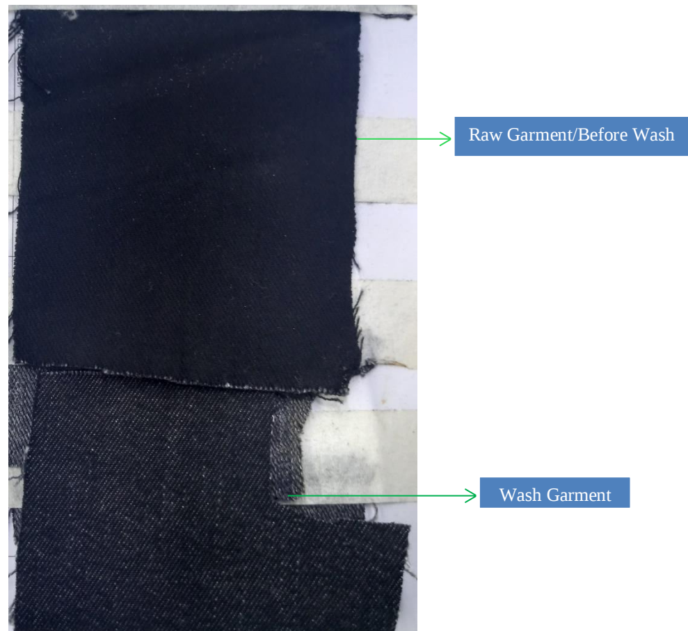
Figure: 3.2 Raw Garment & Enzyme Stone Wash Garment
