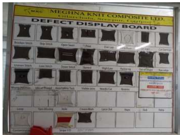
Fig: 2.1 Different types of sewing defects
