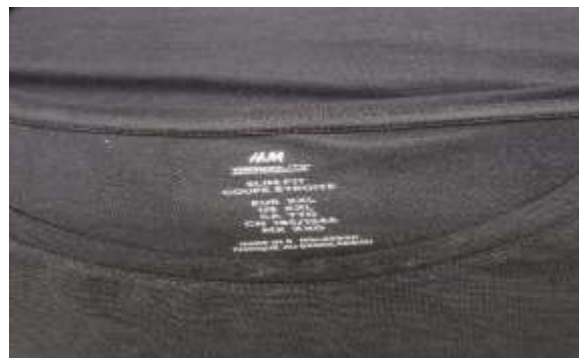
Fig: 2.3 Wrong position of heat seal
